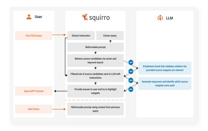
Note: This shows the general logic of the interaction between SquirroGPT and the LLM, it is not a technically precise process-flow diagram.
